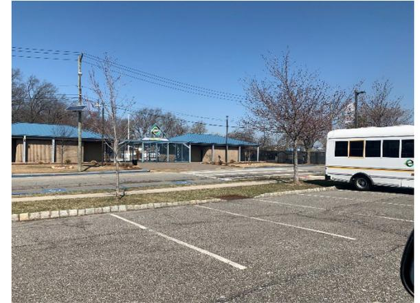
Parking spaces in the center of the parking lot can be converted to porous pavement to capture and infiltrate stormwater runoff from the parking lot. A rain garden can be installed to the north of the building to capture, treat, and infiltrate stormwater runoff from the roof. A tree filter box can be installed around the existing catch basin to intercept stormwater runoff from the parking lot prior to it entering the catch basin.
